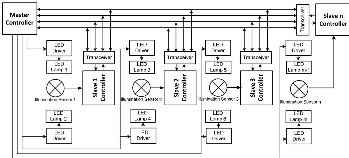
Figure 1. Diagram block of system configuration.
