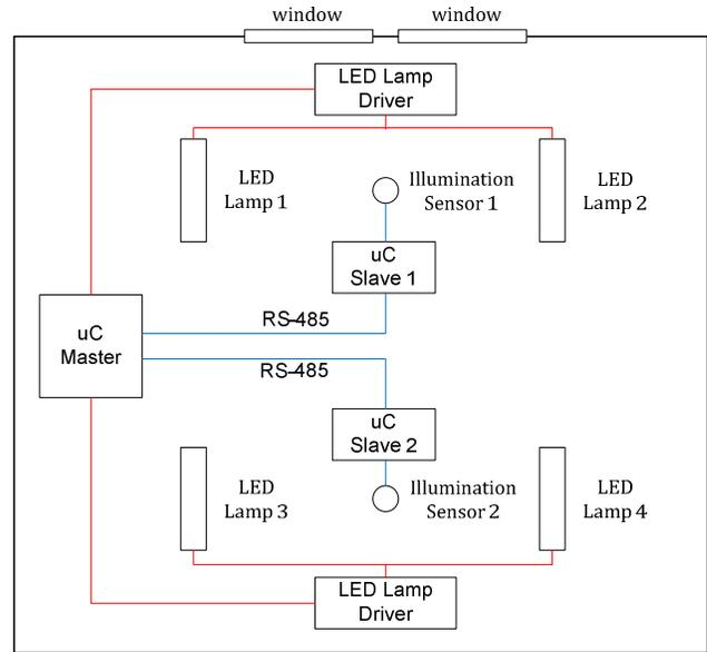
Figure 3. Placement of components.
