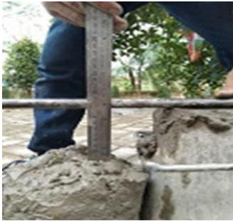
Slump campuran kerang 0% = 95 mm
