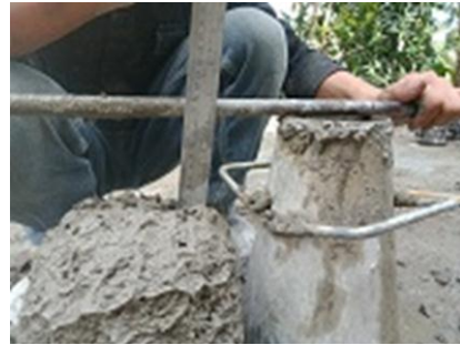
Slump campuran kerang 25% = 90 mm
