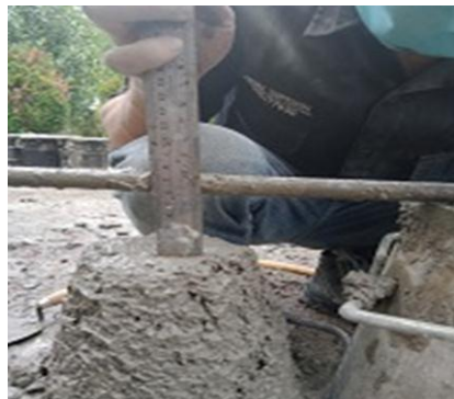
Slump campuran kerang 100% = 58 mm
