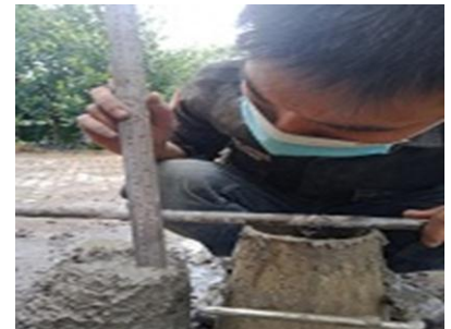
Slump campuran kerang 75% = 74 mm
