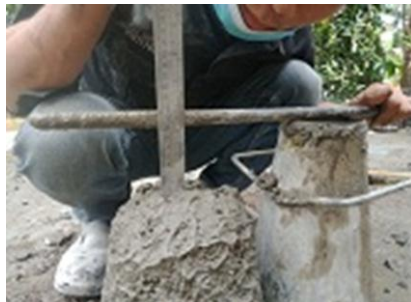
Slump campuran kerang 50% = 80 mm
