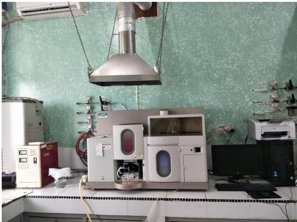
**Gambar 2.** Instrumen AAS (*Atomic Absorption Spectrophotometry*)
