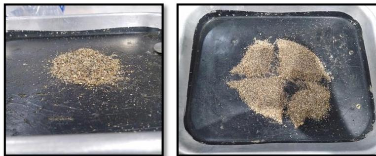
**Gambar 22.** Proses *coning quartering*
