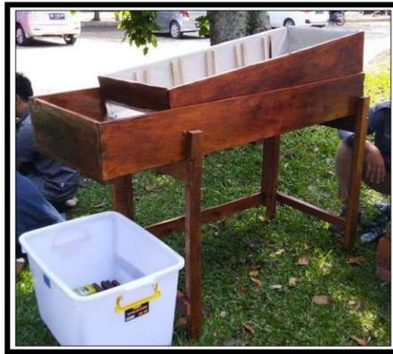
**Gambar 10.** Sluice Box 1.0
