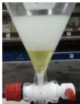
Figure 1. Phase separation results from methyl ester synthesis reactions
