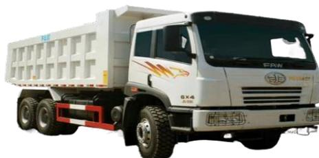
Gambar 2. Alat Angkut (Dump Truck) FAW
