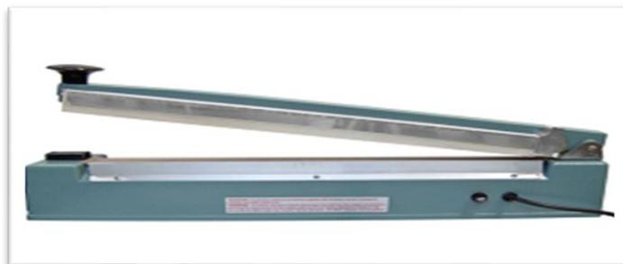
Gambar 6.5 Alat Press Plastik Kemasan
