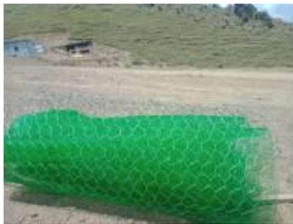
**Gambar 2.4** *Geomat* erosion control
