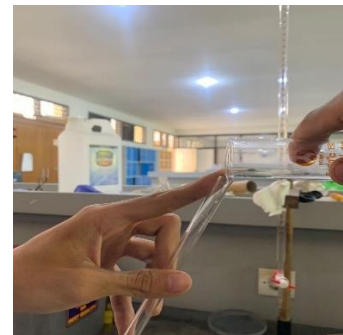
Dimasukkan 15 mL larutan NaOH 1 M kedalam packed column
