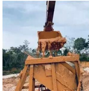
Gambar 4.5 Mesin *Sluice Box*
