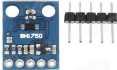
Gambar 8. Sensor intensitas cahaya digital BH1750 Sumber : (Amanda, 2020)
