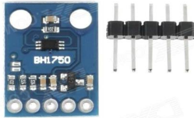
Gambar 8. Sensor intensitas cahaya digital BH1750
