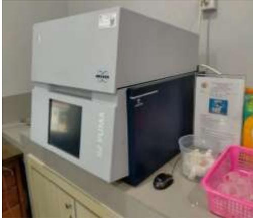
**Gambar** Alat XRF
