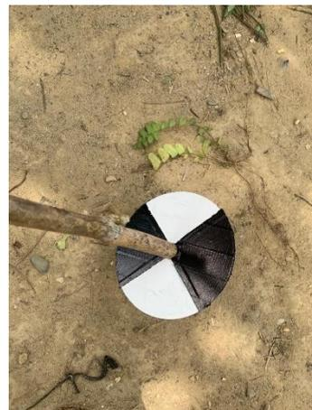
**Gambar 6.** Secchi Disc
