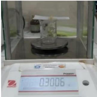
Gambar 39. Timbang sampel uji kadar protein
