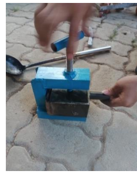
Proses pencetakan paving block
