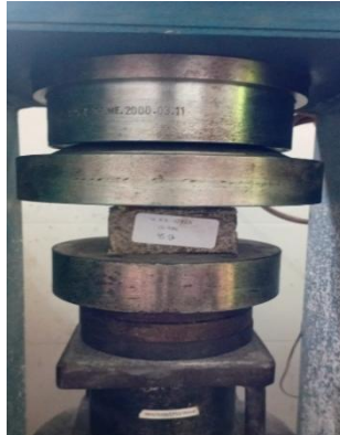
Proses pengujian daya Tekan paving block
